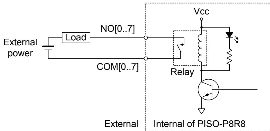
The architecture of PISO-P8SSR8AC (PISO-P8SSR8DC) is similar to the PISO-P8R8. The difference between PISO-P8R8 and PISO-P8SSR8AC (PISO-P8SSR8DC) is that replace the relay by the SSR (solid state relay). The SSR has several special properties as listing: (For more detail specifications please refer to Sec.1.2)
