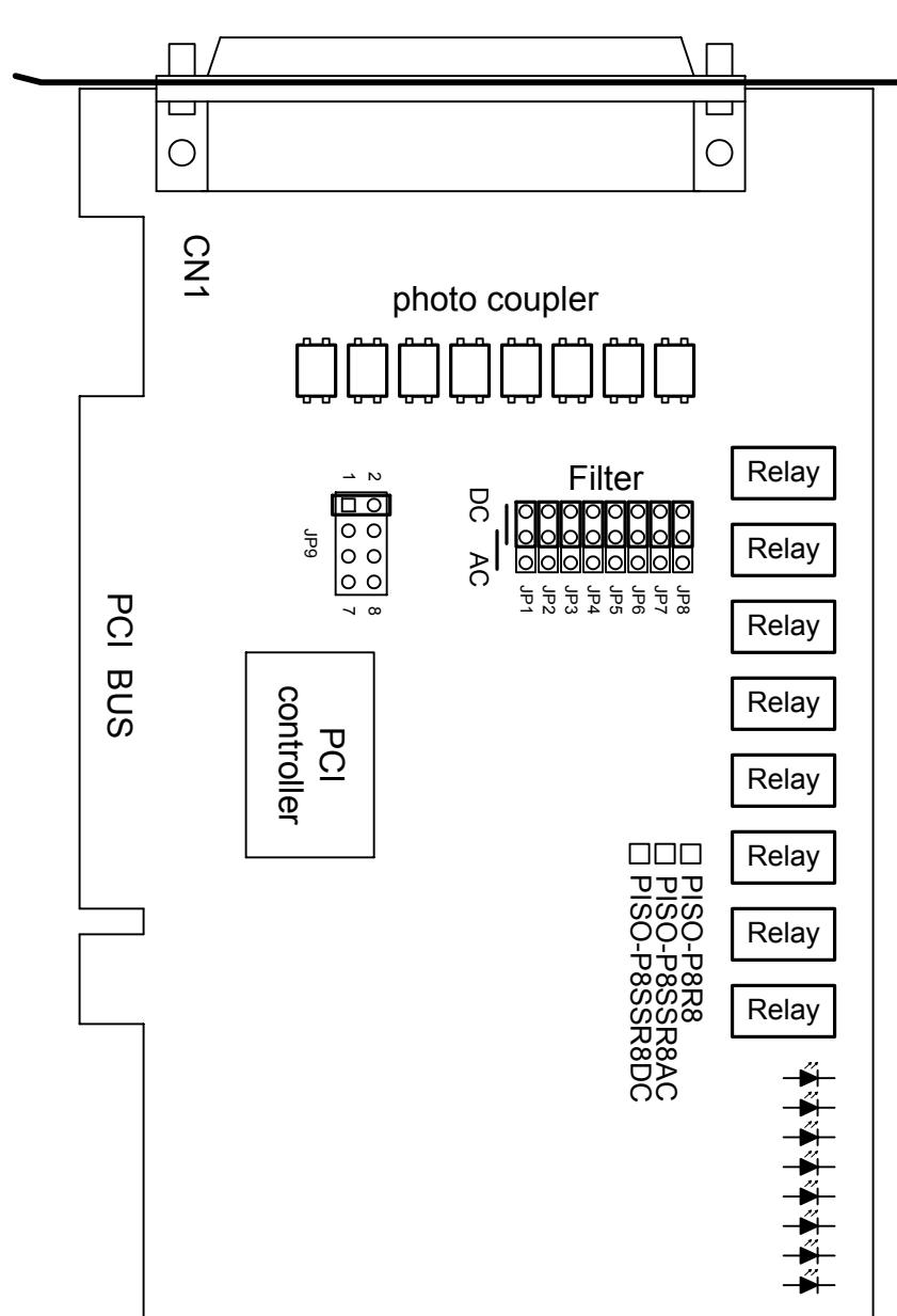
CN1: 8 channels isolated D/I and 8 channels isolated D/O
