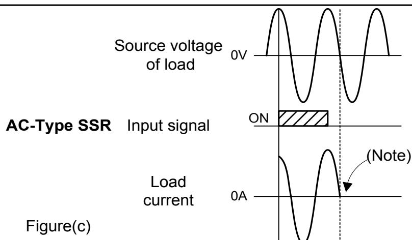
**Note:** The AC-Type SSR is a non zero-crossing SSR. It uses a phototriac coupler to isolate the input from the output. When the input signal is activated, the output immediately turns on, since there is no zero-crossing detector circuit. **The load current is maintained by the triac's latching effect after the input signal is deactivated, until the AC load voltage crosses zero.(Refer to Figure(c).)**
